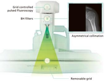
The removable grid provides a further advantage in dose reduction and is especially important when radiation exposure is of particular concern, such as in pediatrics, urology and gynecology.
