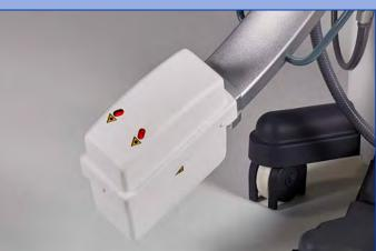
Zero dose centring thanks to laser localisers on X-ray tube and flat panel detector side.
